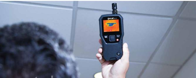
Featuring IGM technology powered by a built-in thermal imaging sensor, the MR176 and MR160 can visually guide you to the precise spot that moisture may be hiding
