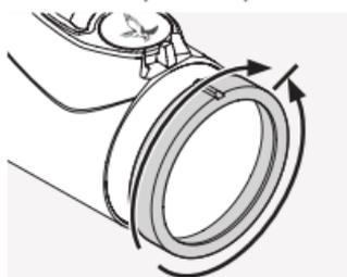
First, turn the diopter adjustment ring fully to the left (counter-clockwise) and then to the right until the reticle is in sharp focus. The adjustment range depends on the individual model.
