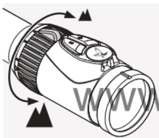
Turn the magnification adjustment ring through up to  $180^\circ$  to obtain the required magnification. The adjustment is continuous. The scale on the adjustment ring makes it easy to see the setting.
