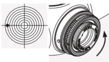
Turn the outer knurled ring on the side turret in the direction of R (counter-clockwise).
