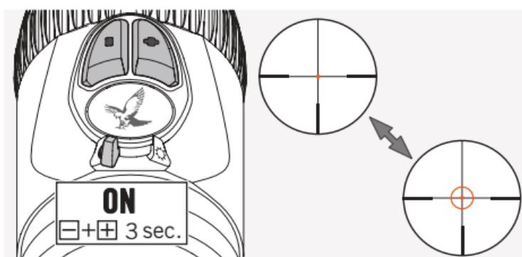
Turn the OFF/DAY/NIGHT switch to the DAY or NIGHT position to switch on the illuminated ring of the FLEXCHANGE 4A-IF reticle. The reticle illumination is now activated. Press the +/- buttons at the same time for 3 seconds to switch on the illuminated ring. Repeat this step to switch the ring off again.
