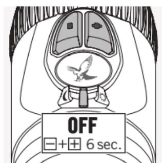
You can deactivate the SWAROLIGHT function by turning the OFF/DAY/NIGHT switch to the central position and pressing the +/- buttons at the same time for 6 seconds. The light will flash twice to confirm that the function is deactivated. You can reactivate the SWAROLIGHT by repeating this step.
