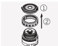
Unscrew the knurled ring from the turret. Remove the knurled ring and the graduated ring (or the marking rings).
